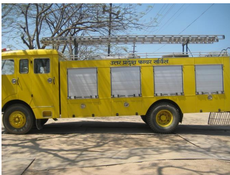
Figure 10: Firefighting Multi-utility vehicle
